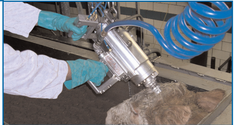
Non-penetrating stunner used with monorail restrainer.
