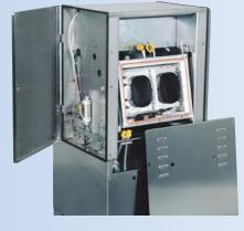
The TS-30 is easily accessible from all sides which helps to reduce maintenance and service time. Tooling dies can be easily changed in 10-15 minutes, without the use of special tools, and are all precisely manufactured by Sipromac according to your tray specifications.
