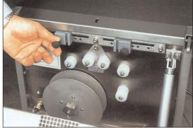
This time saver assists in your packaging process by opening and inflating any brand-name shrink bag or vacuum pouch before your product is placed in the bag. The inflation of the bag, created by the stainless steel blower, greatly improves the ease of
