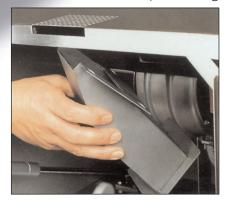
A stainless steel water drip pan at the blower provides for easy disassembly for cleaning. Its construction meets with hygienic standards and complies with all safety requirements.
