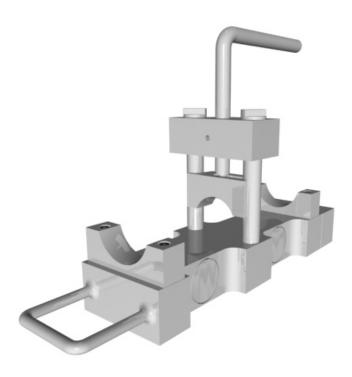
Designed with the oil field in mind, Massload has developed a low cost cable tension monitor sensor that fits a wide variety of cable sizes. This unique design does not require the user to cut any cables, it simply clamps onto the cable.
