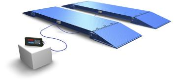
Massload Axle Pad Scales are fully electronic. There are no moving parts to wear out or adjust. Weight is measured using our precision machined, high strength load cells located within the platforms. They are environmentally sealed and virtually indestructible, ensuring years of trouble free operation. The platforms are constructed of heavy-duty structural
