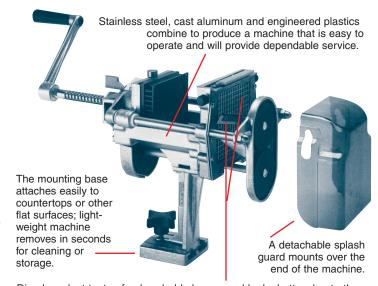
Diced product tastes fresher, holds longer and looks better due to the Easy Dicer's unique double slicing action. Produce is cut twice, once as it passes through the 1/4" or 1/2" slicing grid and then again by the rotating razor sharp blade. This unique "No tears" system locks in flavor, retains juice, increases product yield and gives you mounds of great looking, precision-diced fresh produce in seconds.
