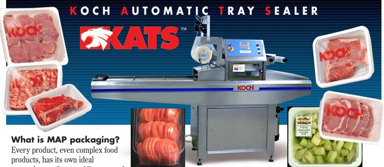
Every product, even complex food products, has its own ideal atmosphere – Oxygen, Nitrogen and Carbon Dioxide. By using a carefully controlled mixture of gases, processors and packers can adjust the atmosphere within a package by using modified atmosphere packaging (MAP). This technology is used to preserve the freshness and extend the shelf-life of products and provides the best way to ensure products are safely packaged in order to reach the consumer in optimum condition.
