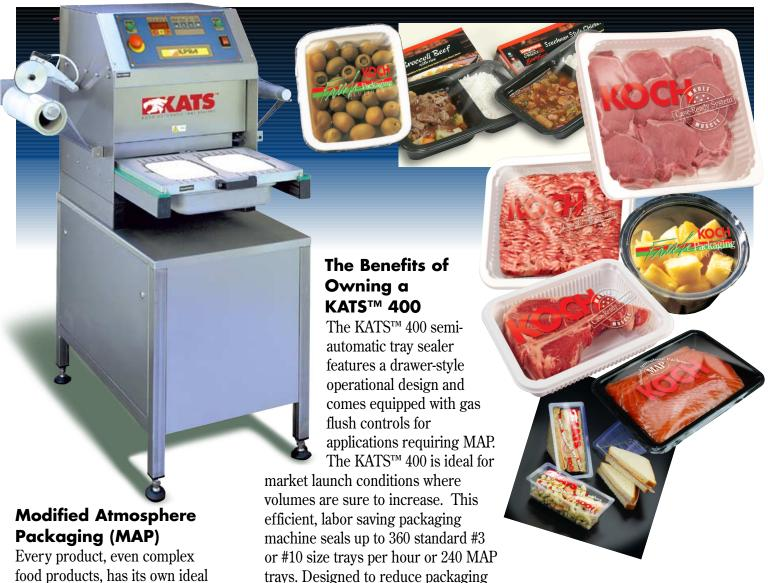
Every product, even complex food products, has its own ideal atmosphere – Oxygen, Nitrogen and Carbon Dioxide. By using a carefully controlled mixture of gases, packers and processors can adjust the atmosphere within a package by using a technology known as modified atmosphere packaging (MAP). This technology is used to preserve the freshness and extend the shelf-life of products and provides the best way to ensure products are safely packaged in order to reach the consumer in optimum condition.
