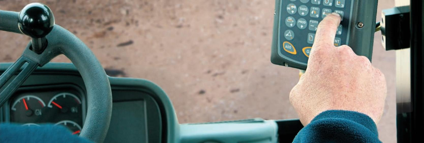
Install the Loadrite Pro on your loader and quickly see for yourself. In addition to its extensive data capabilities, it's also highly accurate, packed with features and simple to use. With other products on the market, loader movement can prevent an accurate reading. The Loadrite Pro is so smart that it can sense a bad lift and advise the operator to perform the lift again – not quite talking back to you, but almost.
